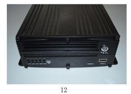
Make sure whether power switch is turned on or turned off, if it is turned on, please use the key, turn the indentation on the "turn off" position.
