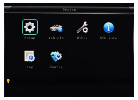
■ Setup setting: includes options of "Base", "User", "Serinal", "PTZ", "GPS", "G-sensor" and "NTP"
