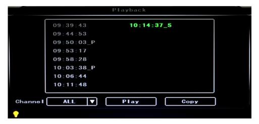
There are video date in the menu, it will display the vide time after enter the date, choose the playback time range as needed, press "Play" or click the interface "Playback "button to replay the video. Said is power outage file suffix "\_P", suffix "\_S" indicates an alarm trigger video files.
