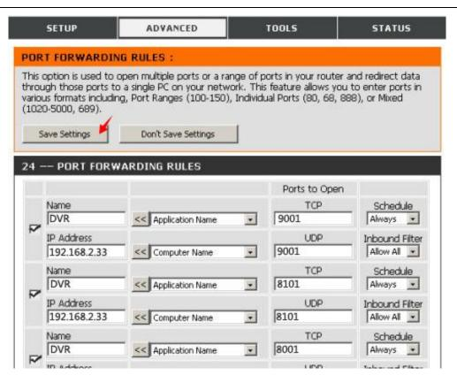
✓ After the port mapping settings, find the "**IP Address**" in the WAN, the IP Address is your CMS server IP. login the server IP on the CMS client to access.
